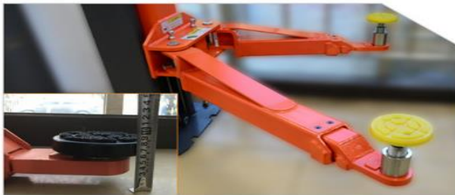
2 & 3 stages ultra-low arms, for the low chassis sport car, strength 20% higher
